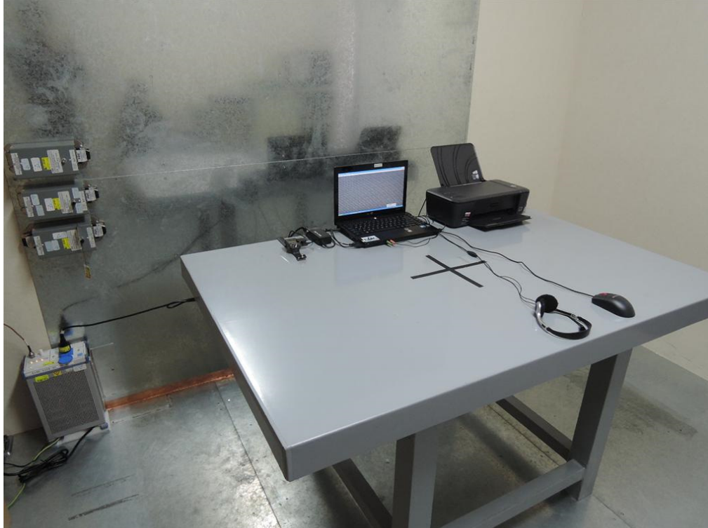
Photograph 6: Set-up for for Mains Conducted testing Front
