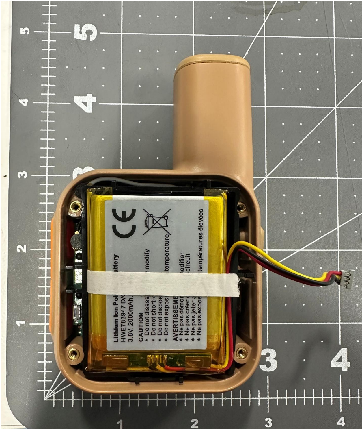
Inside View of Front Housing w/ battery and battery carrier in place
