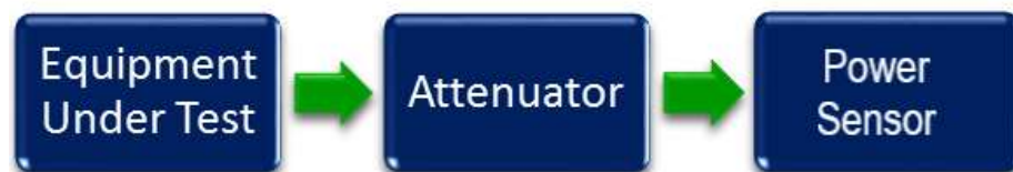
Figure 1. Output RF power Test Setup
