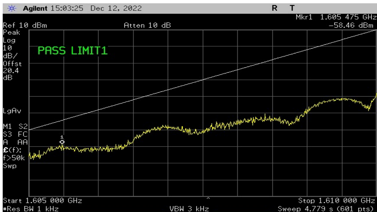
Plot 23- Low Channel – Test Limit 25.216 (f)(g) – Discrete Emissions
