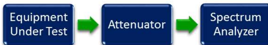
Figure 3: Spurious Emission at Antenna Terminal Test setup
