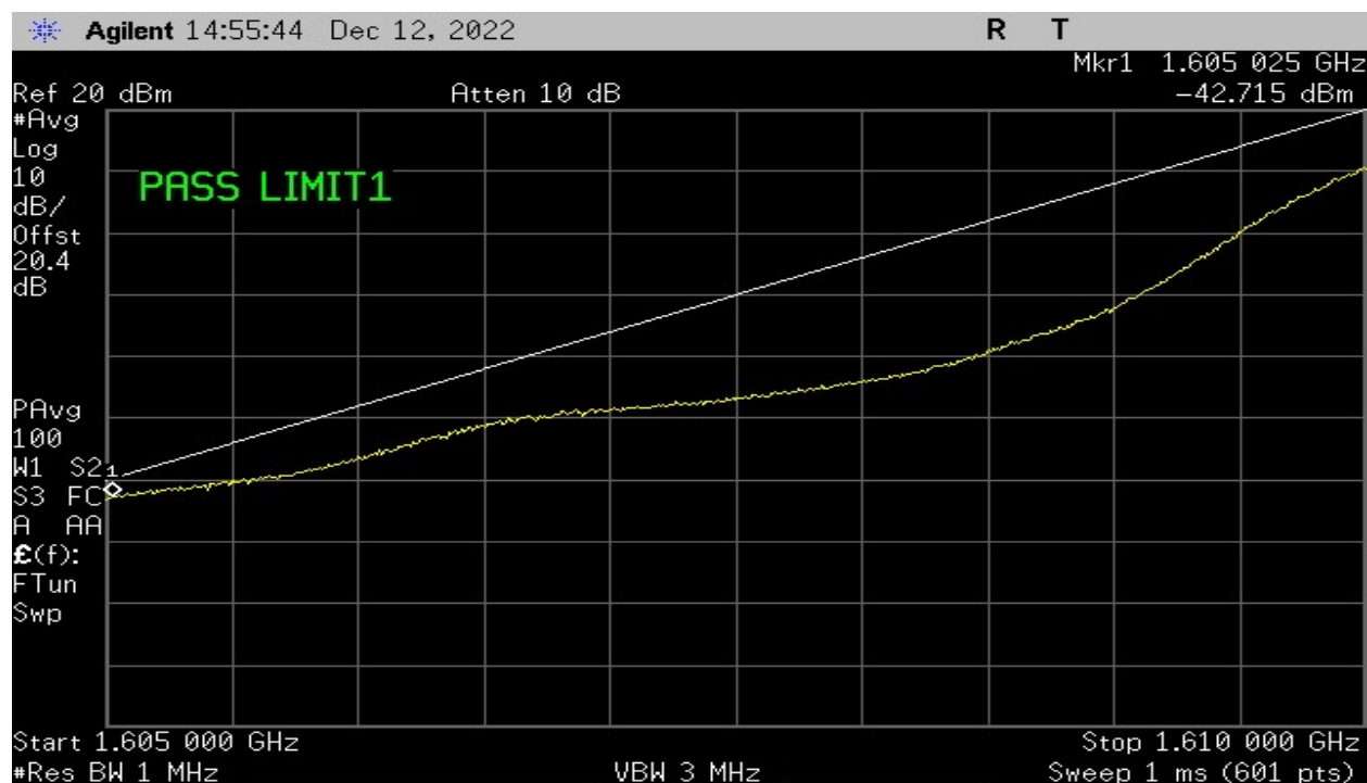
Plot 25- Low Channel – Test Limit 25.216 (f)(g)
