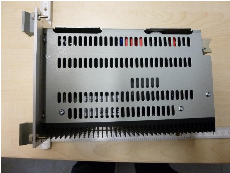
Photo 3: Power supply module
