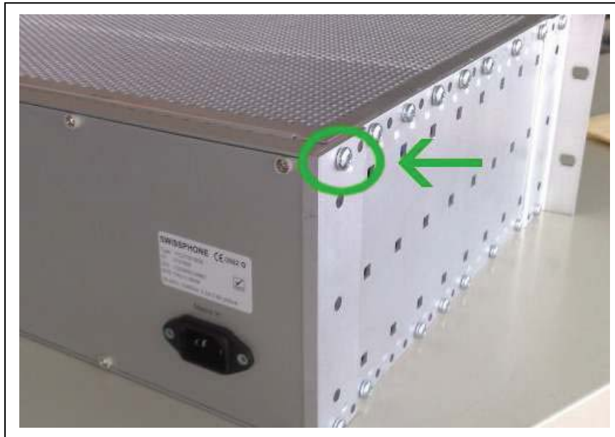
Fig. 6-1: Grounding point at ITC2100-BOS
