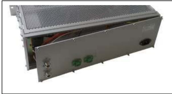
Fig. 6-13: Removing the ITC2100-BOS rear panel
