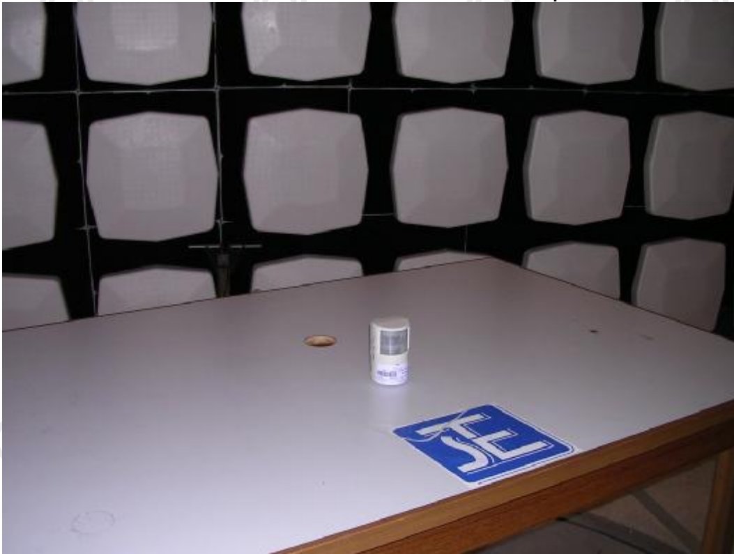
Measurement of Radiated Emission Test Set Up
