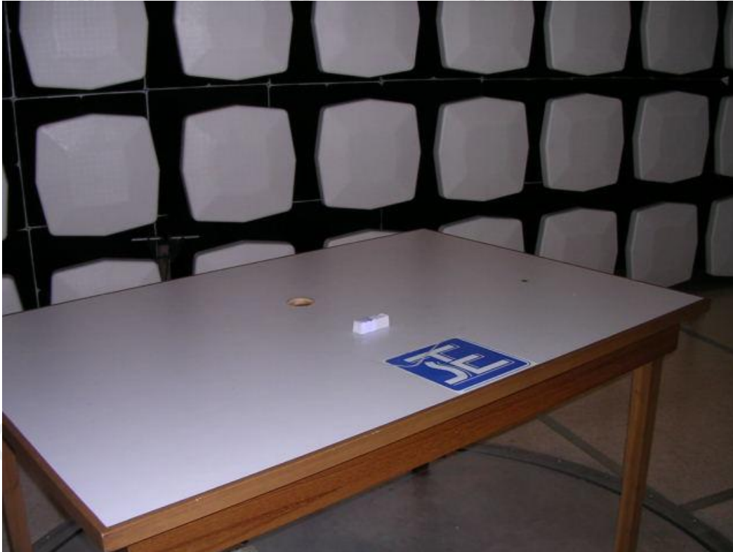
Measurement of Radiated Emission Test Set Up
