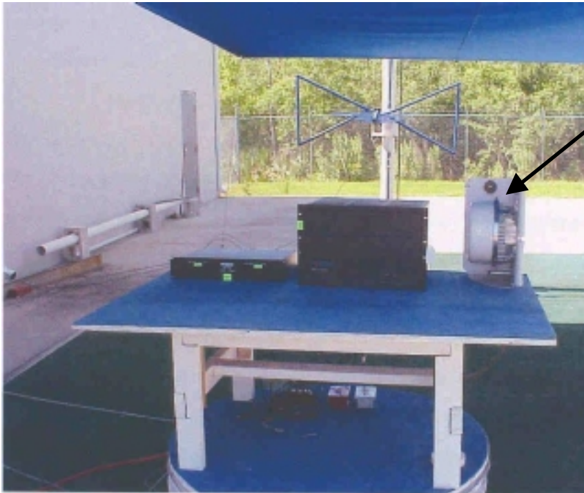
Sector ODU and Antenna
