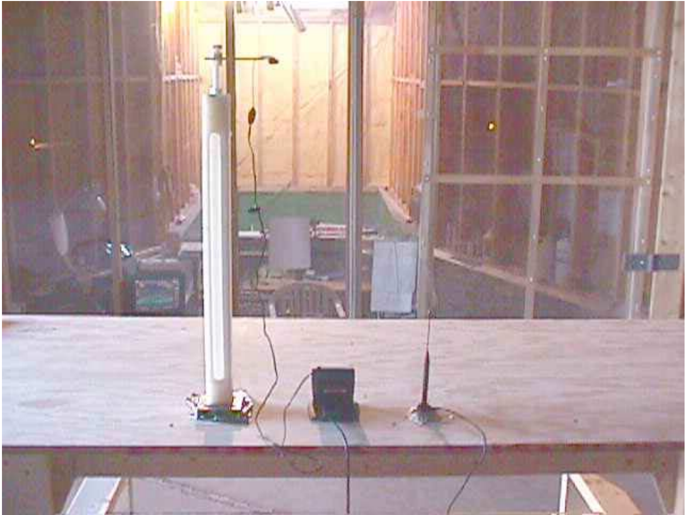
Test Configuration # 1: EUT in Cradle with Headset
