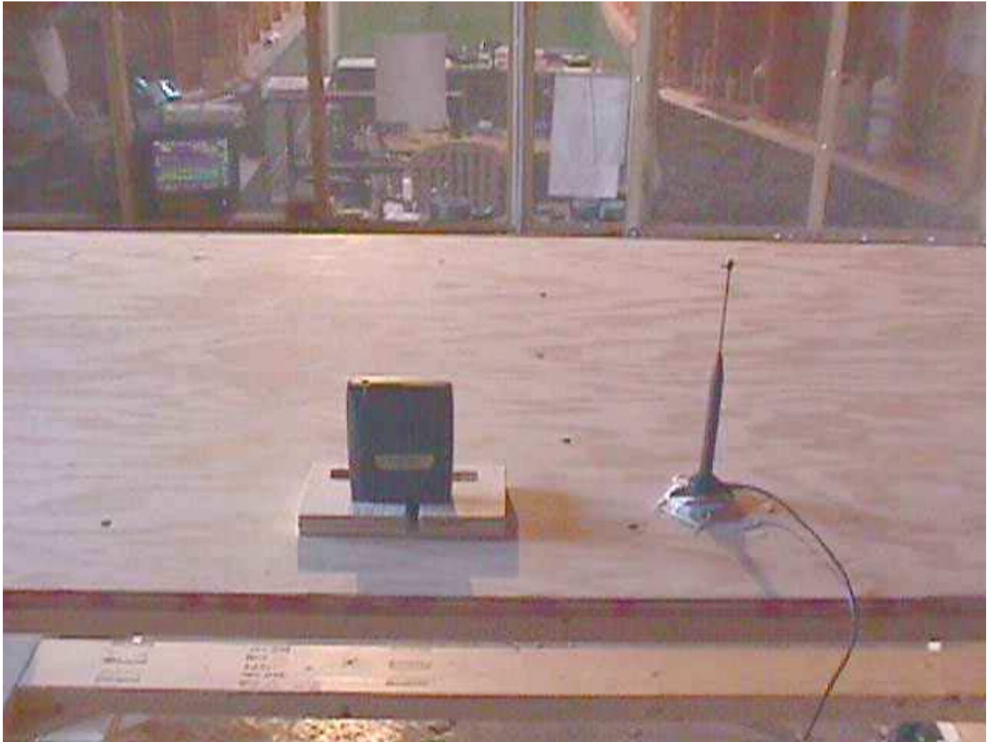
Test Configuration # 4: EUT Standalone (Upright Position)
