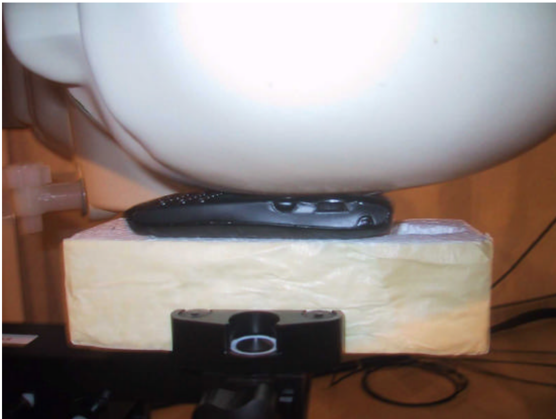
SAR set-up photos for head configuration: antenna close to (top) and far (bottom - 40mm distance) from the holder
