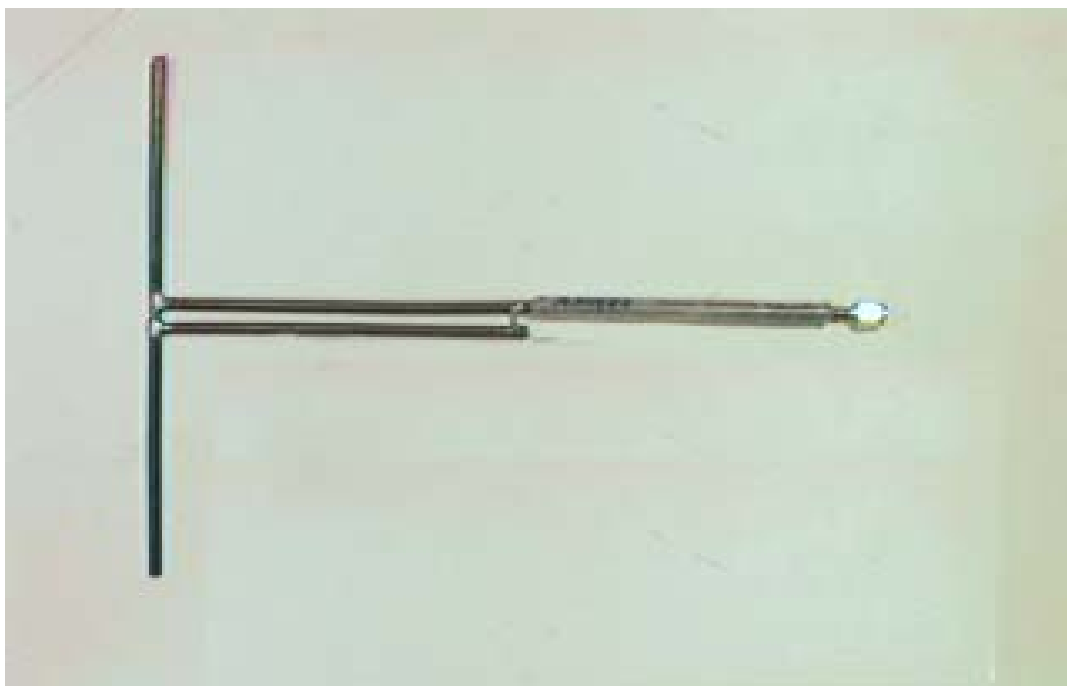
Reference Dipole Antenna Used for ERP Measurement
