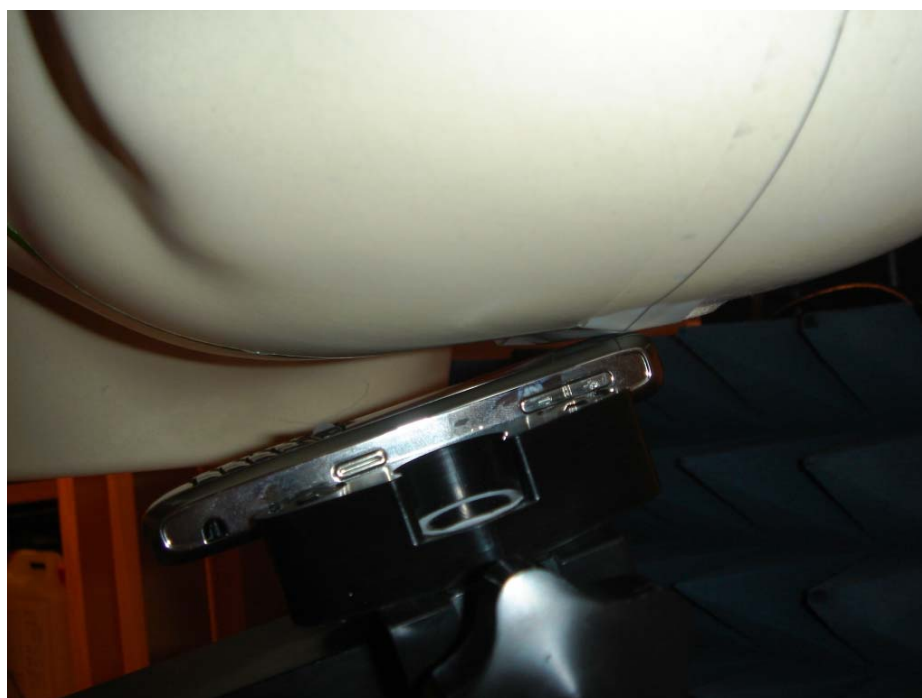
Figure E6. Head configuration (Left Tilted)
