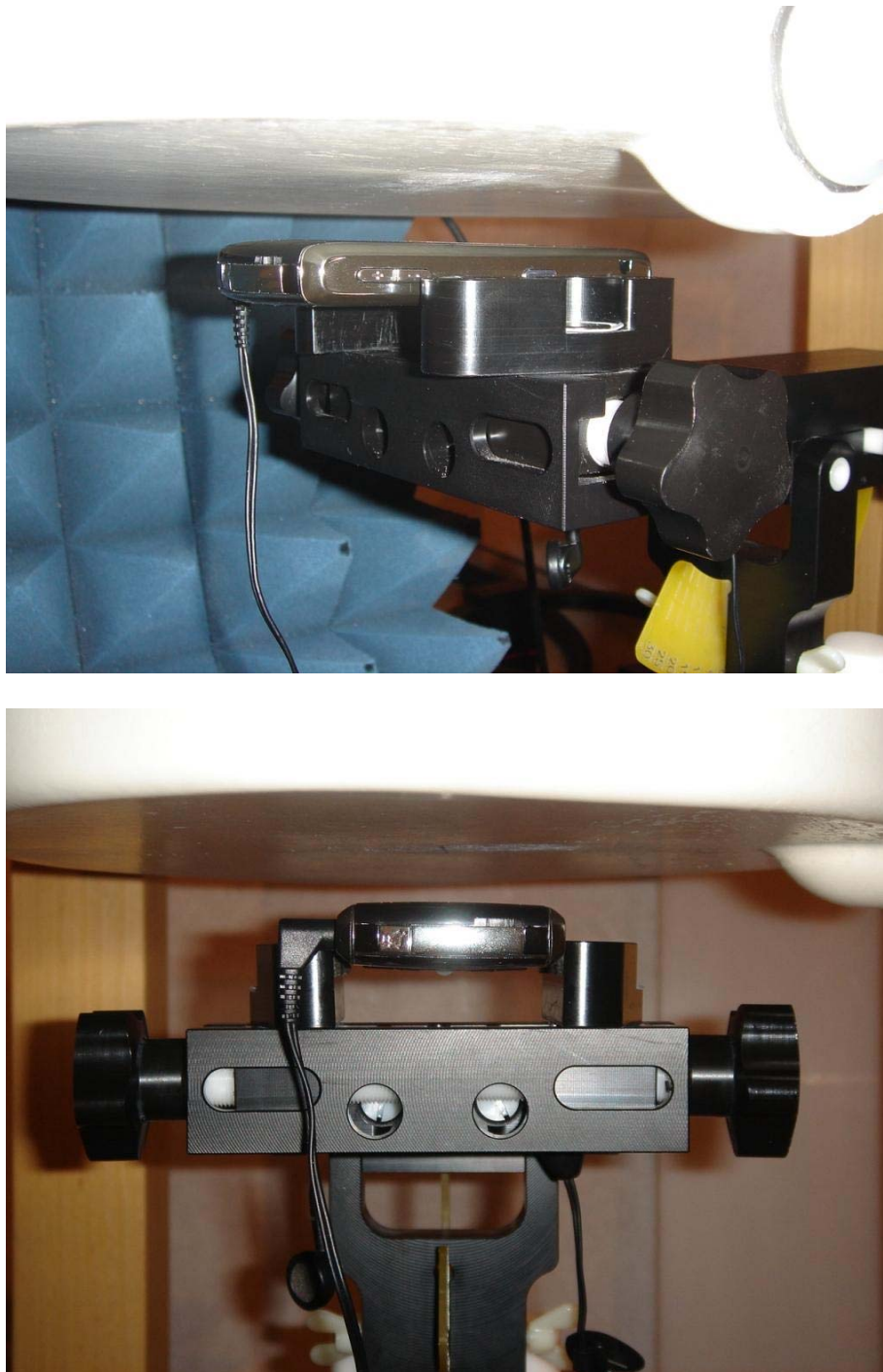
Figure E12. Body-worn configuration (No Holster, 15 mm away, with Mono Headset and Bluetooth connected, back facing phantom)
