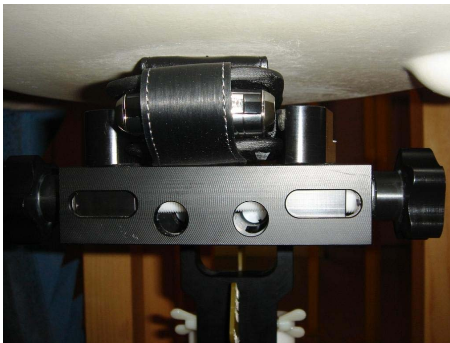
Figure E7. Body-worn configuration (Leather Holster, front facing phantom)
