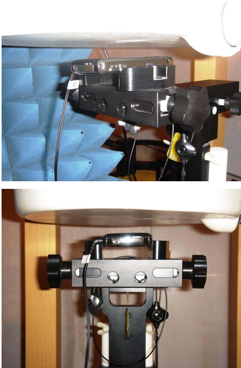
Figure E13. Body-worn configuration (No Holster, 15 mm away, with Stereo Headset and Bluetooth connected, back facing phantom)
