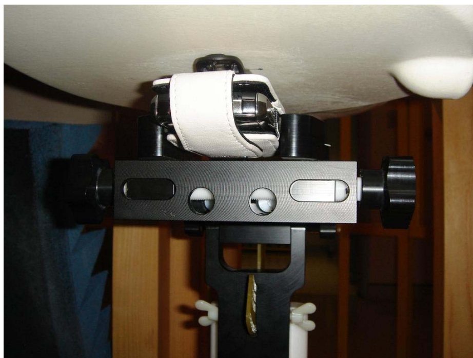
Figure E10. Body-worn configuration (Leather Swivel Holster, back facing phantom)
