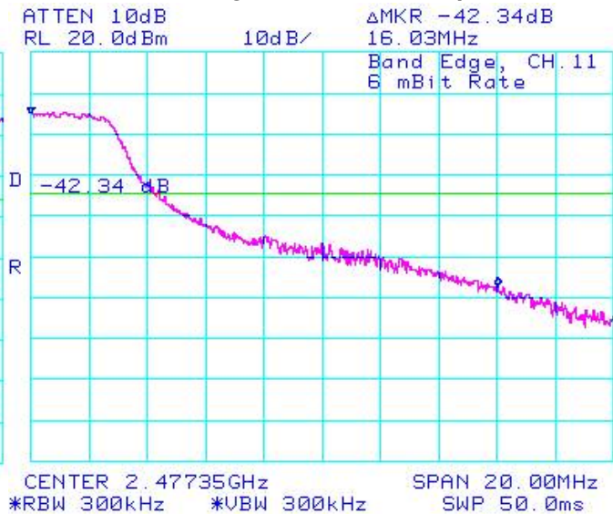
Figure 4-10: Band Edge Compliance
