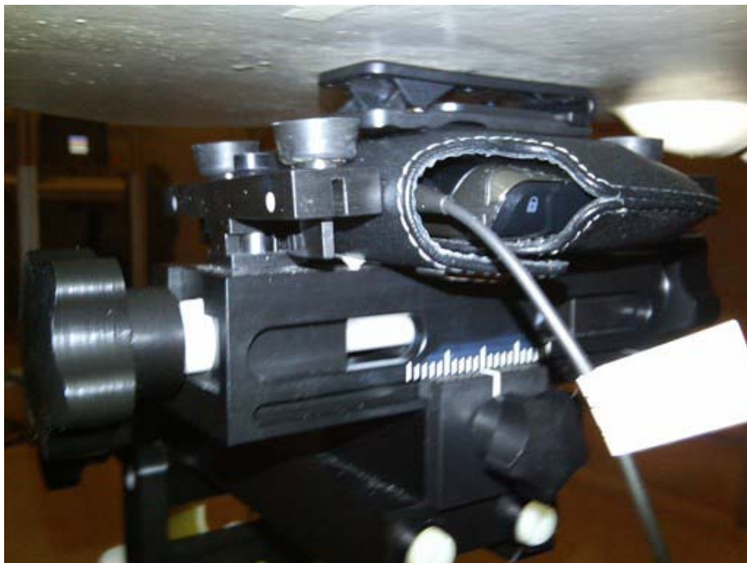
Figure E15. Body-worn configuration (Horizontal Holster, headset 3, back facing phantom)
