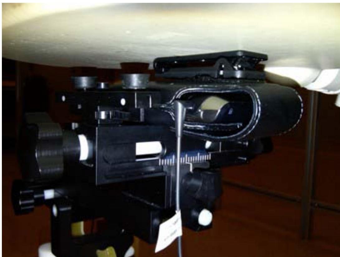
Figure E9. Body-worn configuration (Vertical Holster , headset 3, back facing phantom)
