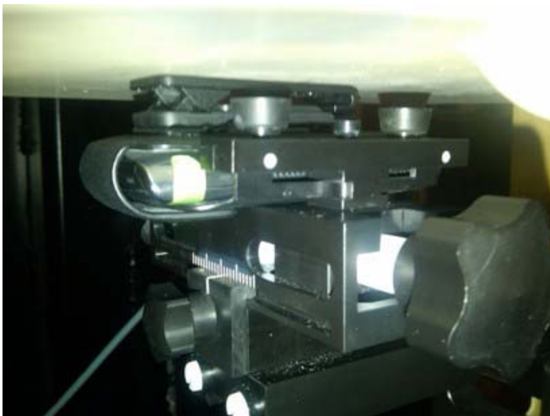
Figure E6. Body-worn configuration (Vertical Holster, back facing phantom)
