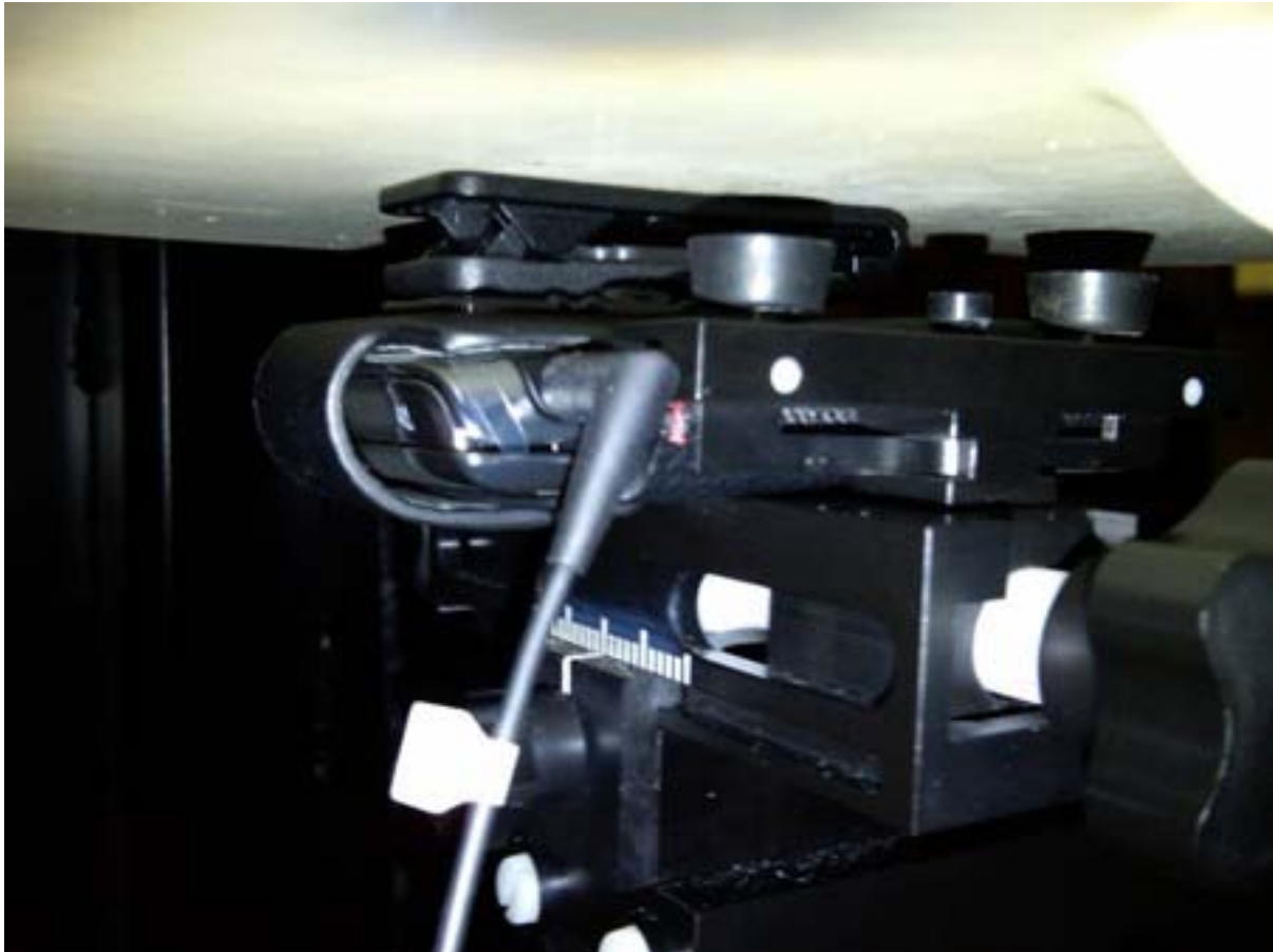
Figure E10. Body-worn configuration (Vertical Holster , headset 2, back facing phantom)
