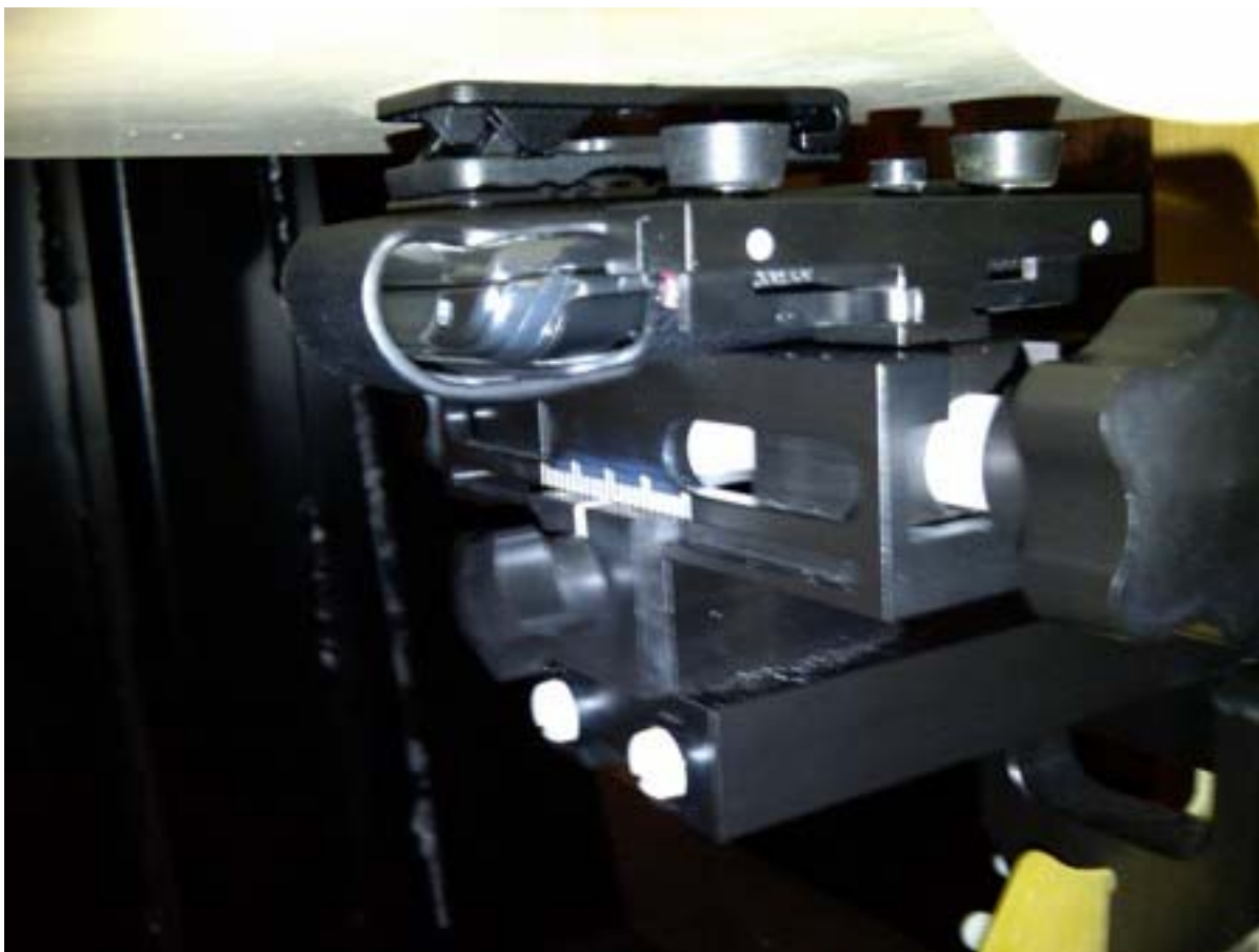
Figure E12. Body-worn configuration (Vertical Holster, front facing phantom)
