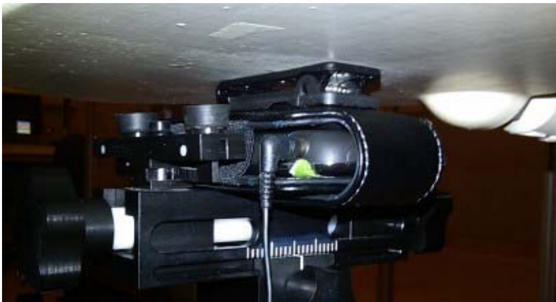
Figure E7. Body-worn configuration (Vertical Holster , headset 1, back facing phantom)
