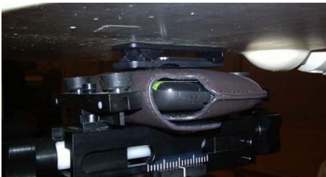
Figure E15. Body-worn configuration (Horizontal Holster, front facing phantom)
