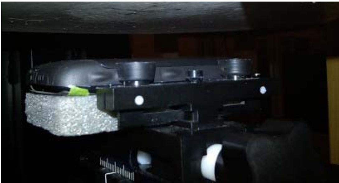
Figure E16. Body-worn configuration (No Holster, 25 mm away, back facing phantom)
