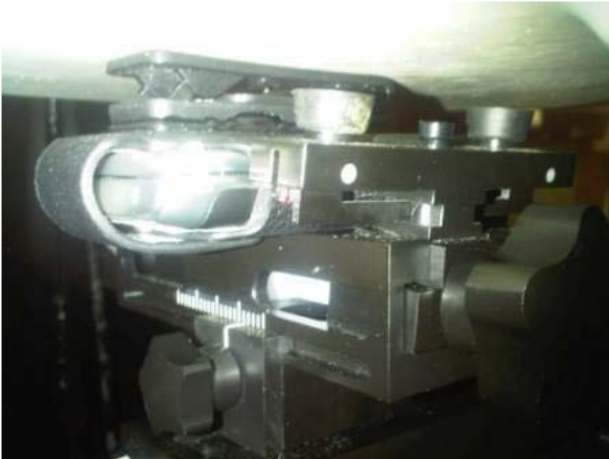
Figure E14. Body-worn configuration (Vertical Holster, front facing phantom)
