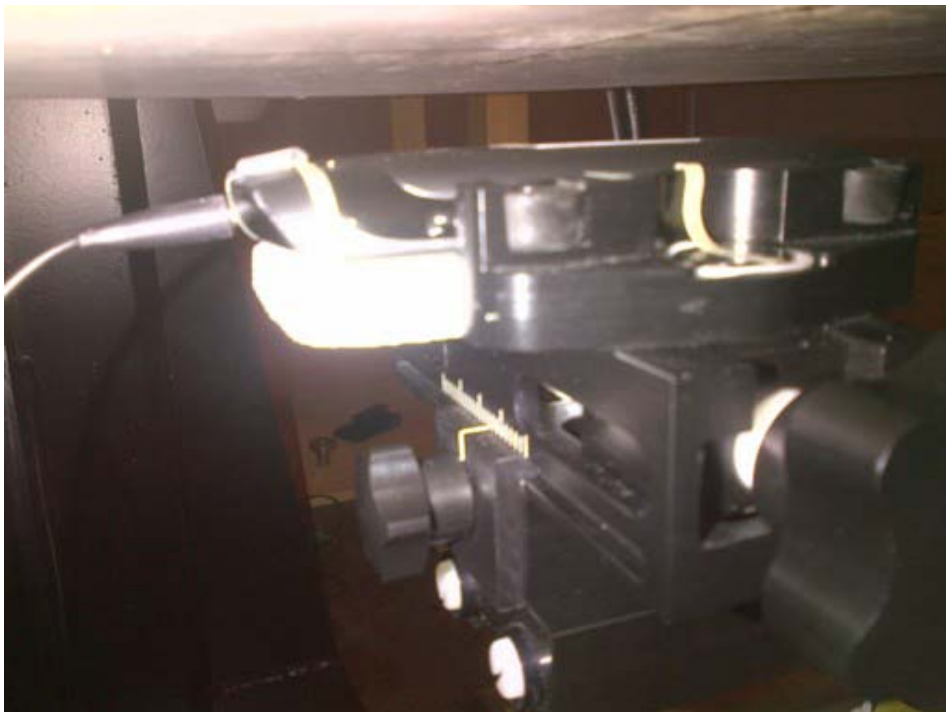
Figure E9. Body-worn configuration (No Holster, headset, back 15mm away)
