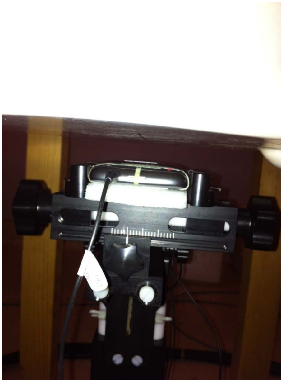
Figure E9. Body-worn configuration (No Holster, headset, back 15mm away)
