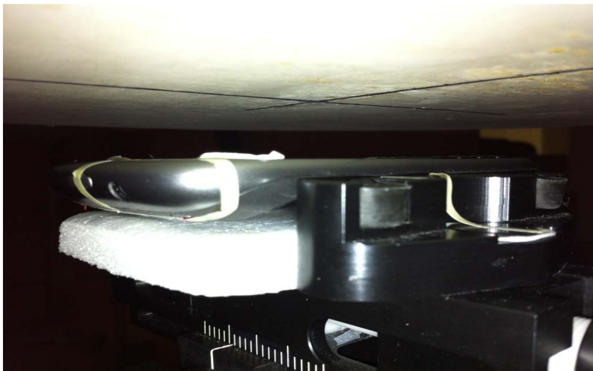
Figure E7. Body-worn configuration (No Holster, front side 20mm away)
