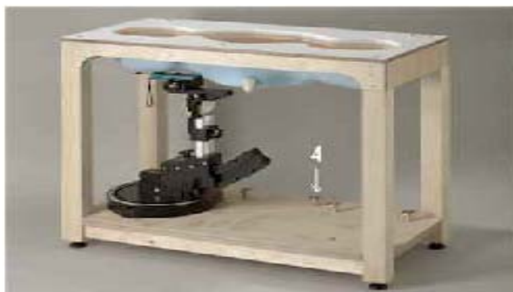
Figure 5.0-1 SAM Twin Phantom
