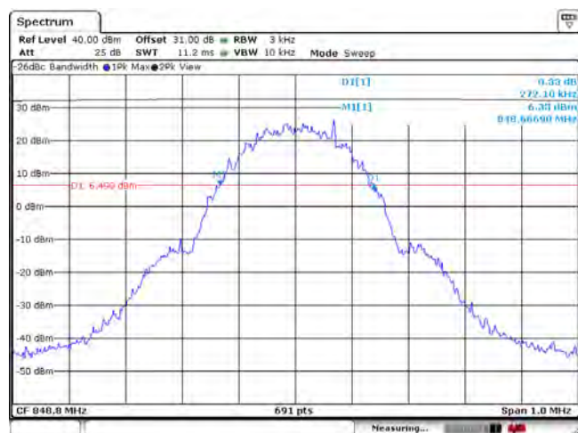
Figure 1-15a: -26dBc bandwidth, GSM850 band High Channel in GSM mode
