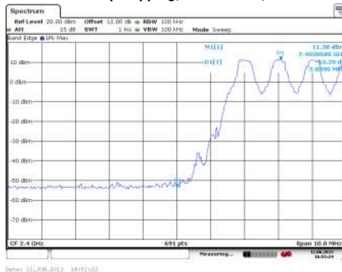
Figure 2-37: Band Edge Compliance Freq. Hopping, Static PBRS, DH5
