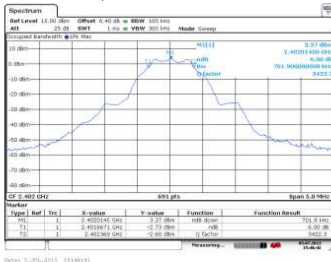
Figure 2-59: 6 dB Bandwidth LE, Channel 0
