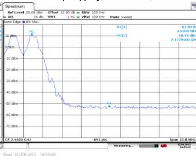
Figure 2-38: Band Edge Compliance Freq. Hopping, Static PBRS, DH5
