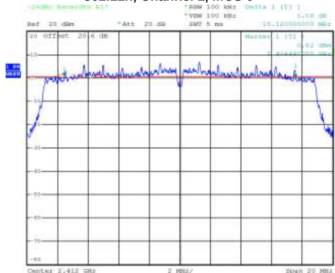
Figure 3-7: 6 dB Bandwidth 802.11n, Channel 1, MCS 0
