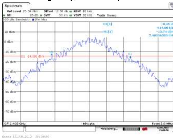
Figure 2-1: 20 dB Bandwidth Single freq., Static PBRs, DH5
