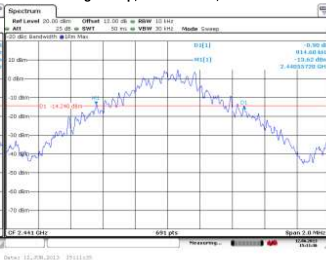
Figure 2-2: 20 dB Bandwidth Single freq., Static PBRs, DH5
