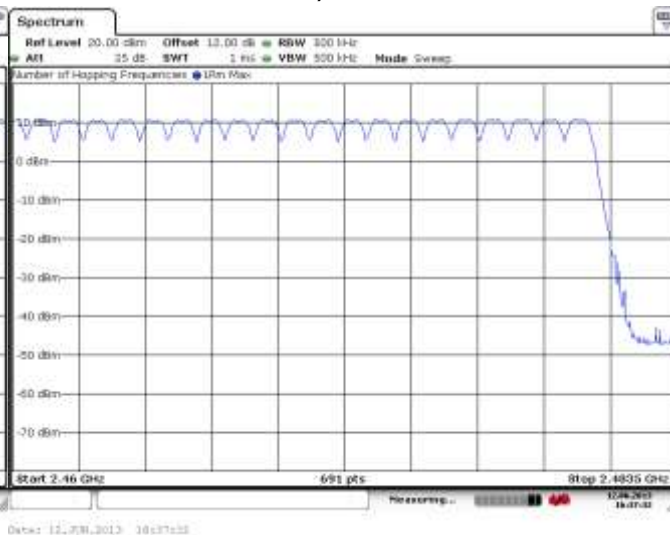
Figure 2-16: Number of Hopping Frequencies Static PBRS, DH5
