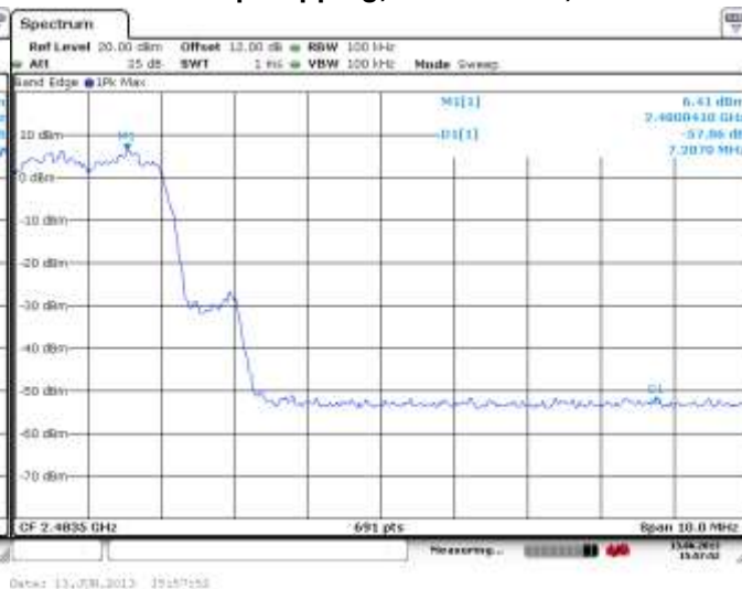
Figure 2-46: Band Edge Compliance Freq. Hopping, Static PBRS, 3-DH5
