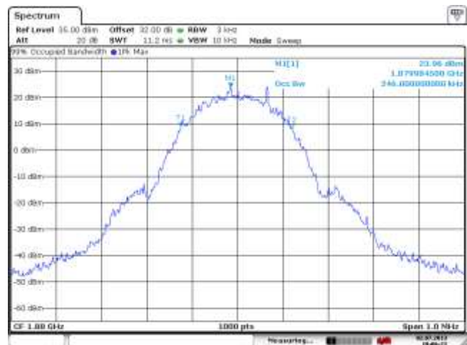
Figure 1-22a: Occupied Bandwidth, PCS1900 Middle Channel in GSM mode
