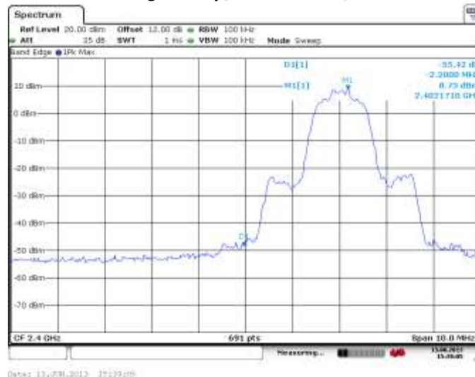
Figure 2-39: Band Edge Compliance Single Freq., Static PBRs, 2-DH5
