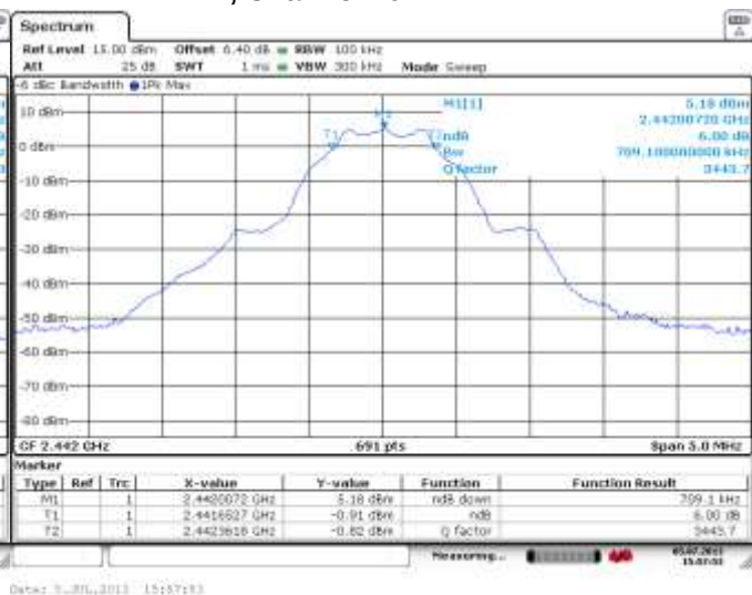
Figure 2-60: 6 dB Bandwidth LE, Channel 20
