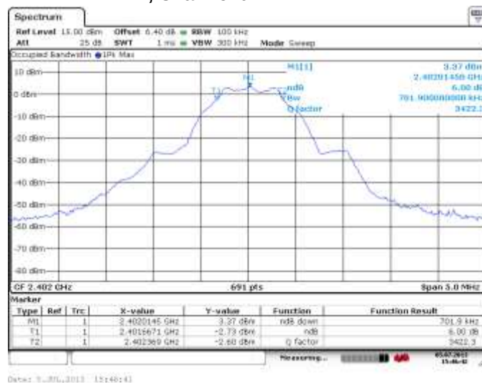
Figure 2-59: 6 dB Bandwidth LE, Channel 0
