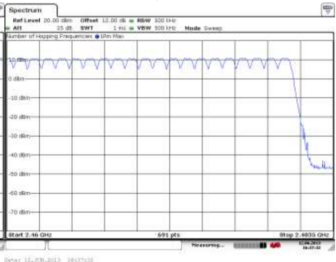
Figure 2-16: Number of Hopping Frequencies Static PBRS, DH5
