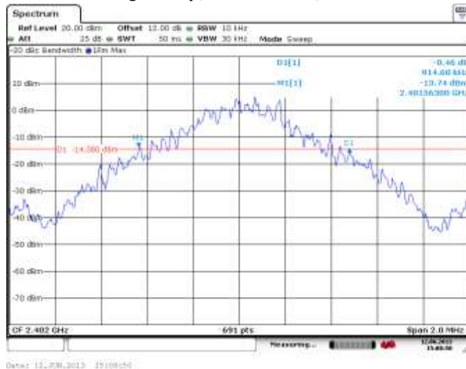
Figure 2-1: 20 dB Bandwidth Single freq., Static PBRS, DH5
