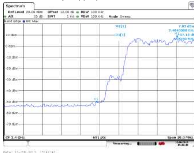
Figure 2-41: Band Edge Compliance Freq. Hopping, Static PBRs, 2-DH5
