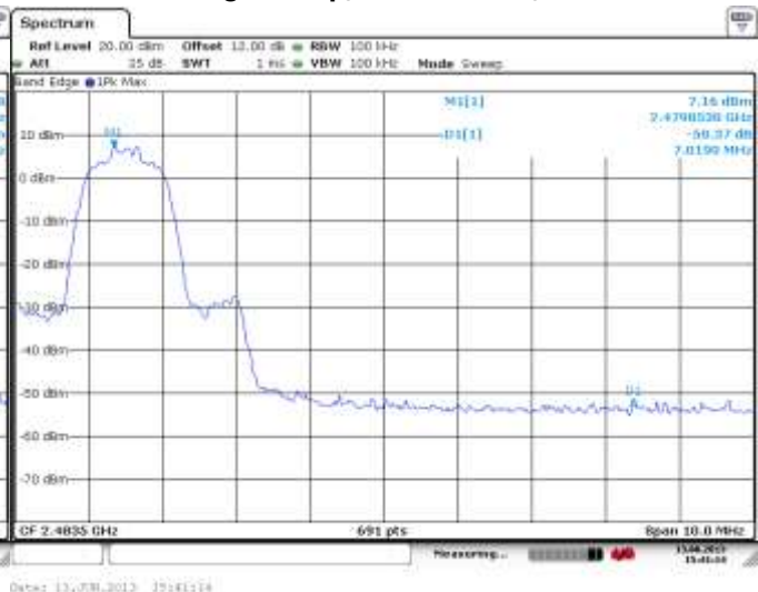
Figure 2-40: Band Edge Compliance Single Freq., Static PBRs, 2-DH5
