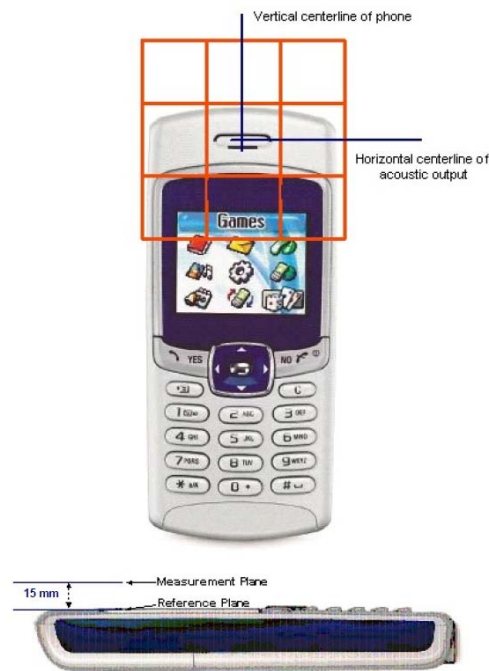
Figure 5.5-2: WD reference plane for RF emission measurement
