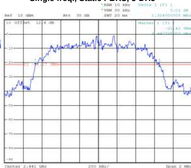
Figure 2-8: 20 dB Bandwidth Single freq., Static PBRs, 3-DH5
