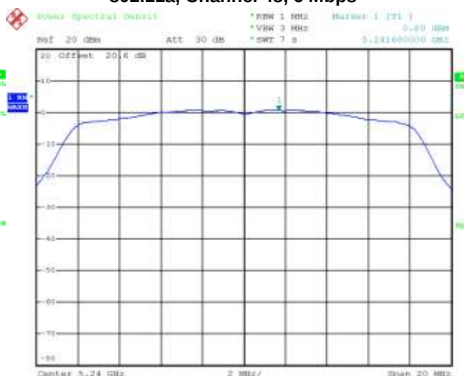
Figure 4-23: Peak Power Spectral Density 802.11a, Channel 48, 6 Mbps
