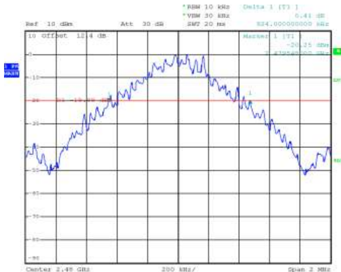
Figure 2-3: 20 dB Bandwidth Single freq., Static PBRs, DH5
