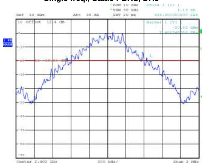
Figure 2-1: 20 dB Bandwidth Single freq., Static PBRS, DH5
