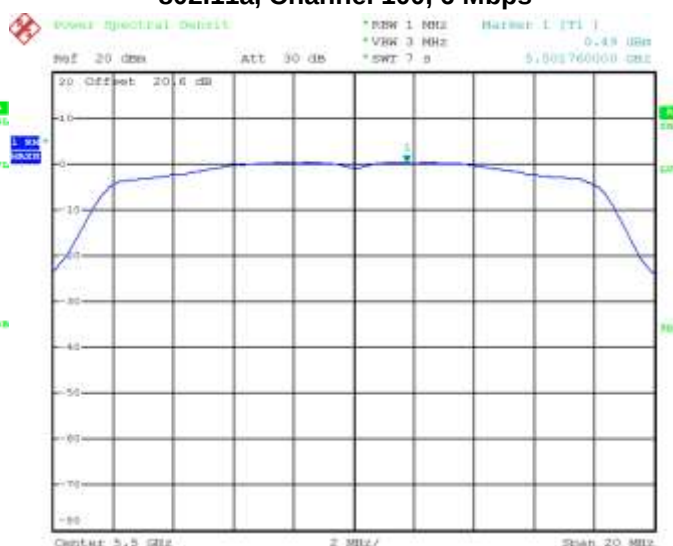
Figure 4-25: Peak Power Spectral Density 802.11a, Channel 100, 6 Mbps
