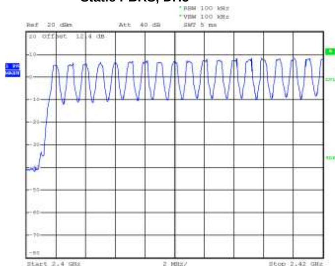
Figure 2-13: Number of Hopping Frequencies Static PBRS, DH5
