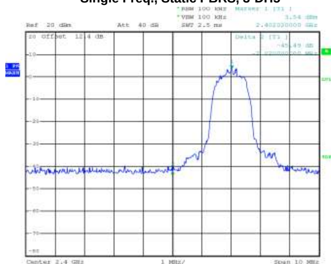
Figure 2-43: Band Edge Compliance Single Freq., Static PBRS, 3-DH5
