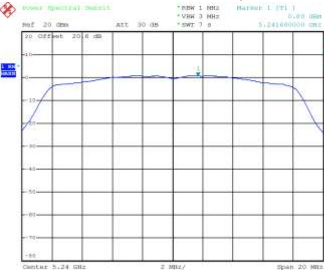
Figure 4-23: Peak Power Spectral Density 802.11a, Channel 48, 6 Mbps
