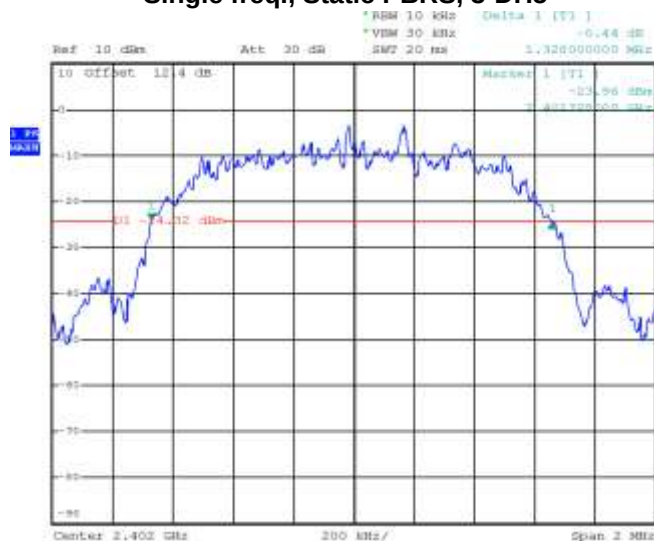
Figure 2-9: 20 dB Bandwidth Single freq., Static PBRs, 3-DH5
