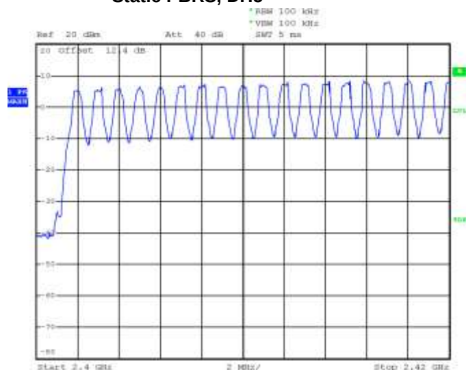
Figure 2-13: Number of Hopping Frequencies Static PBRS, DH5
