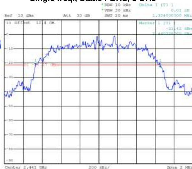
Figure 2-8: 20 dB Bandwidth Single freq., Static PBRs, 3-DH5
