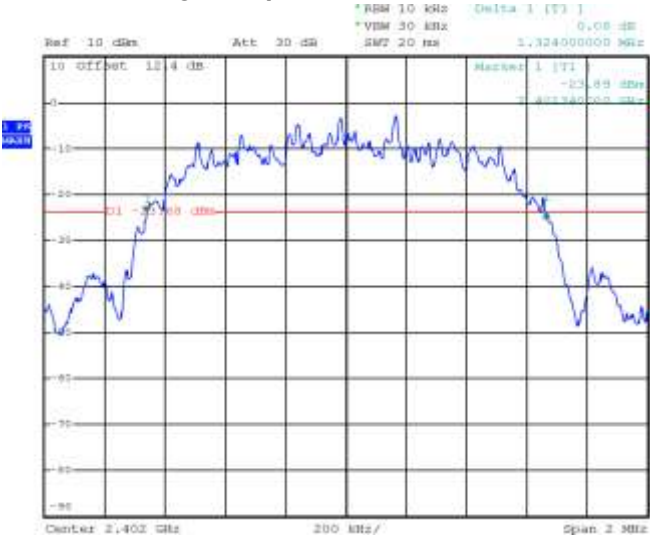
Figure 2-4: 20 dB Bandwidth Single freq., Static PBRS, 2-DH5
