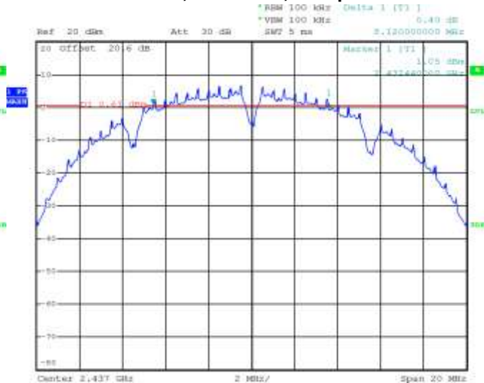
Figure 3-2: 6 dB Bandwidth 802.11b, Channel 6, 1 Mbps
