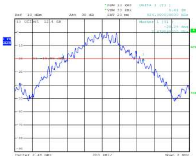
Figure 2-3: 20 dB Bandwidth Single freq., Static PBRs, DH5
