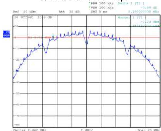
Figure 3-3: 6 dB Bandwidth 802.11b, Channel 11, 1 Mbps
