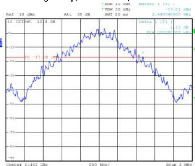
Figure 2-2: 20 dB Bandwidth Single freq., Static PBRS, DH5
