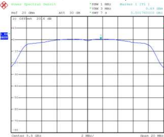
Figure 4-25: Peak Power Spectral Density 802.11a, Channel 100, 6 Mbps
