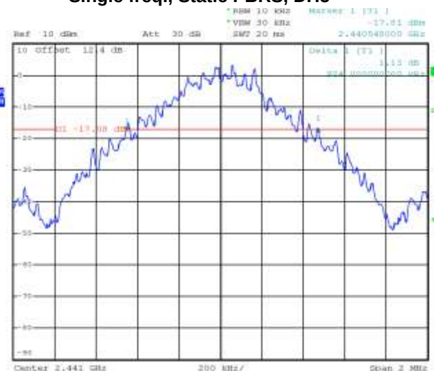
Figure 2-2: 20 dB Bandwidth Single freq., Static PBRS, DH5
