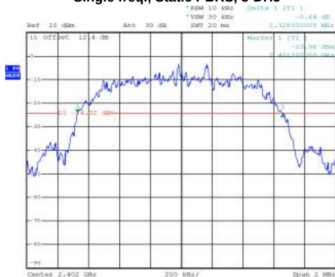
Figure 2-9: 20 dB Bandwidth Single freq., Static PBRs, 3-DH5
