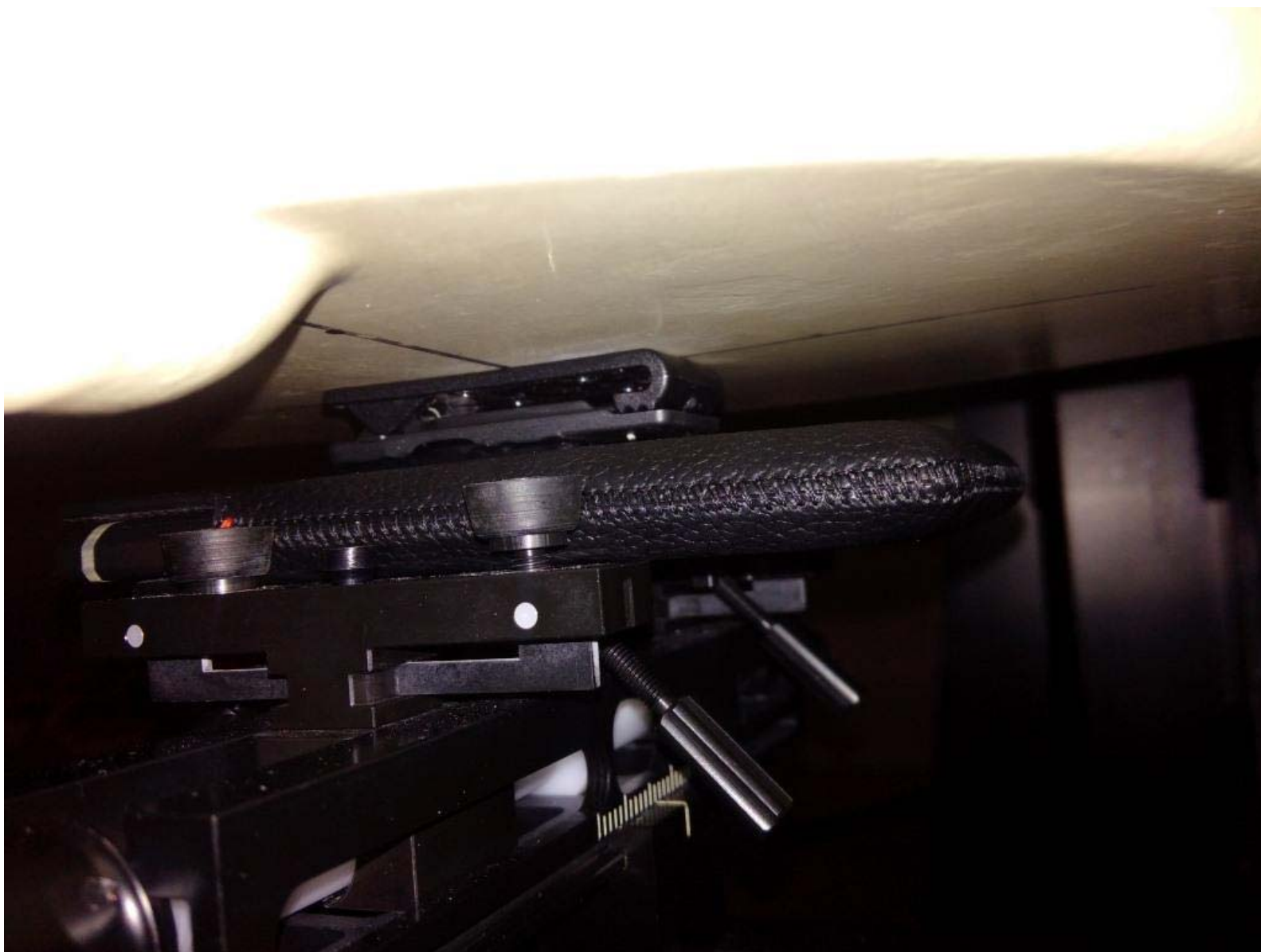
Figure E15. Body-worn configuration (Holster, back)
