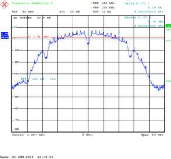
Figure 6-4: 6 dB Bandwidth Primary, 802.11g, Channel 1, 6 Mbps
