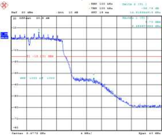
Figure 6-24: Band Edge Compliance Secondary, 802.11n, Channel 11, MCS 0
