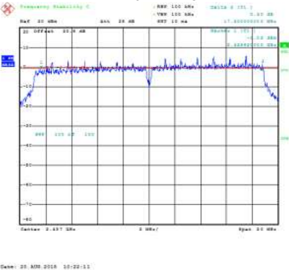
Figure 6-15: 6 dB Bandwidth Secondary, 802.11g, Channel 11, 6 Mbps
