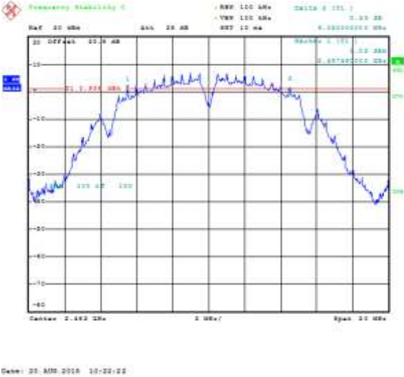
Figure 6-16: 6 dB Bandwidth Secondary, 802.11n, Channel 1, MCS 0
