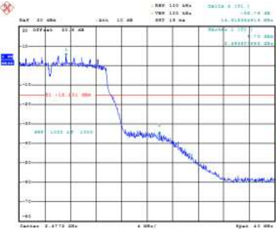
Figure 6-24: Band Edge Compliance Primary, 802.11n, Channel 11, MCS 0
