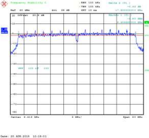
Figure 6-3: 6 dB Bandwidth Primary, 802.11b, Channel 11, 1 Mbps
