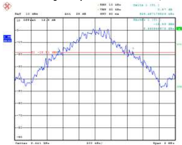
Figure 5-2: 20 dB Bandwidth Single freq. CH 39 Static PBRS, DH5
