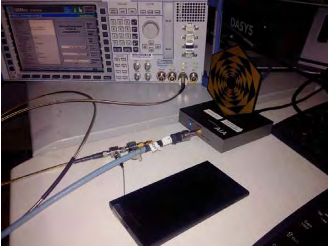
Figure C3 – MIF measurement setup
