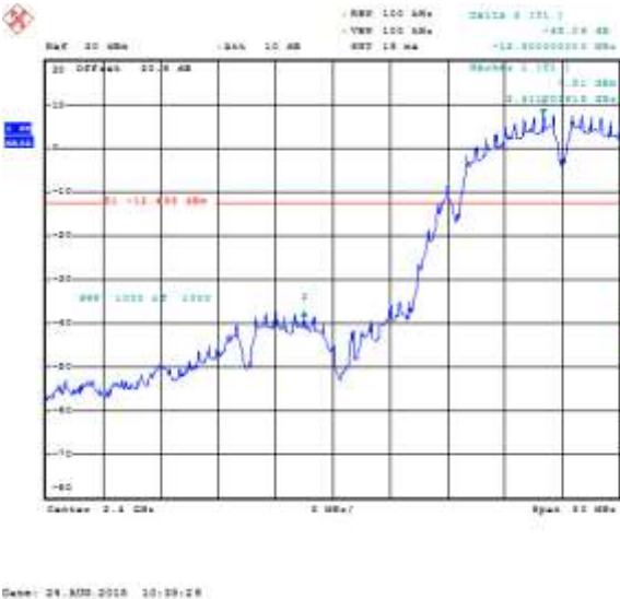
Figure 6-19: Band Edge Compliance Primary, 802.11b, Channel 1, 1 Mbps
