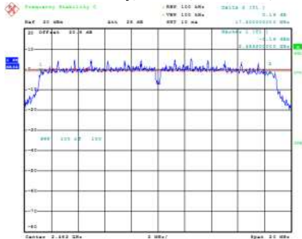
Figure 6-9: 6 dB Bandwidth Primary, 802.11n, Channel 11, MCS 0
