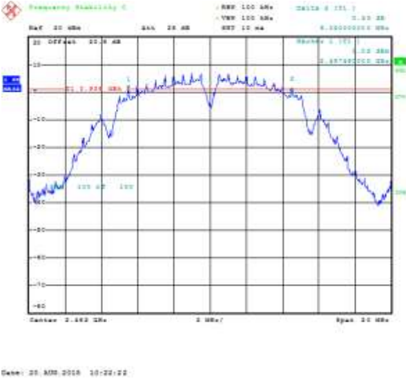
Figure 6-16: 6 dB Bandwidth Secondary, 802.11n, Channel 1, MCS 0
