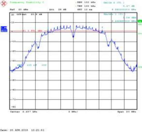
Figure 6-13: 6 dB Bandwidth Secondary, 802.11g, Channel 1, 6 Mbps
