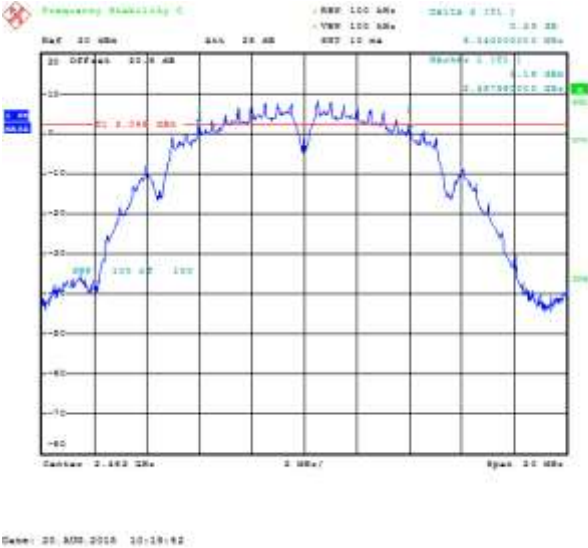
Figure 6-7: 6 dB Bandwidth Primary, 802.11n, Channel 1, MCS 0
