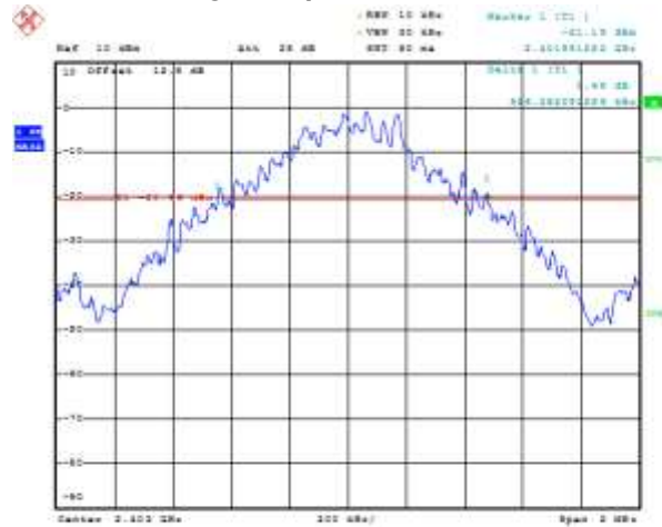
Figure 5-1: 20 dB Bandwidth Single freq. CH 0 Static PBRS, DH5
