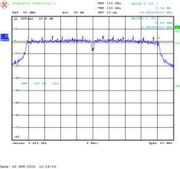
Figure 6-8: 6 dB Bandwidth Primary, 802.11n, Channel 6, MCS 0
