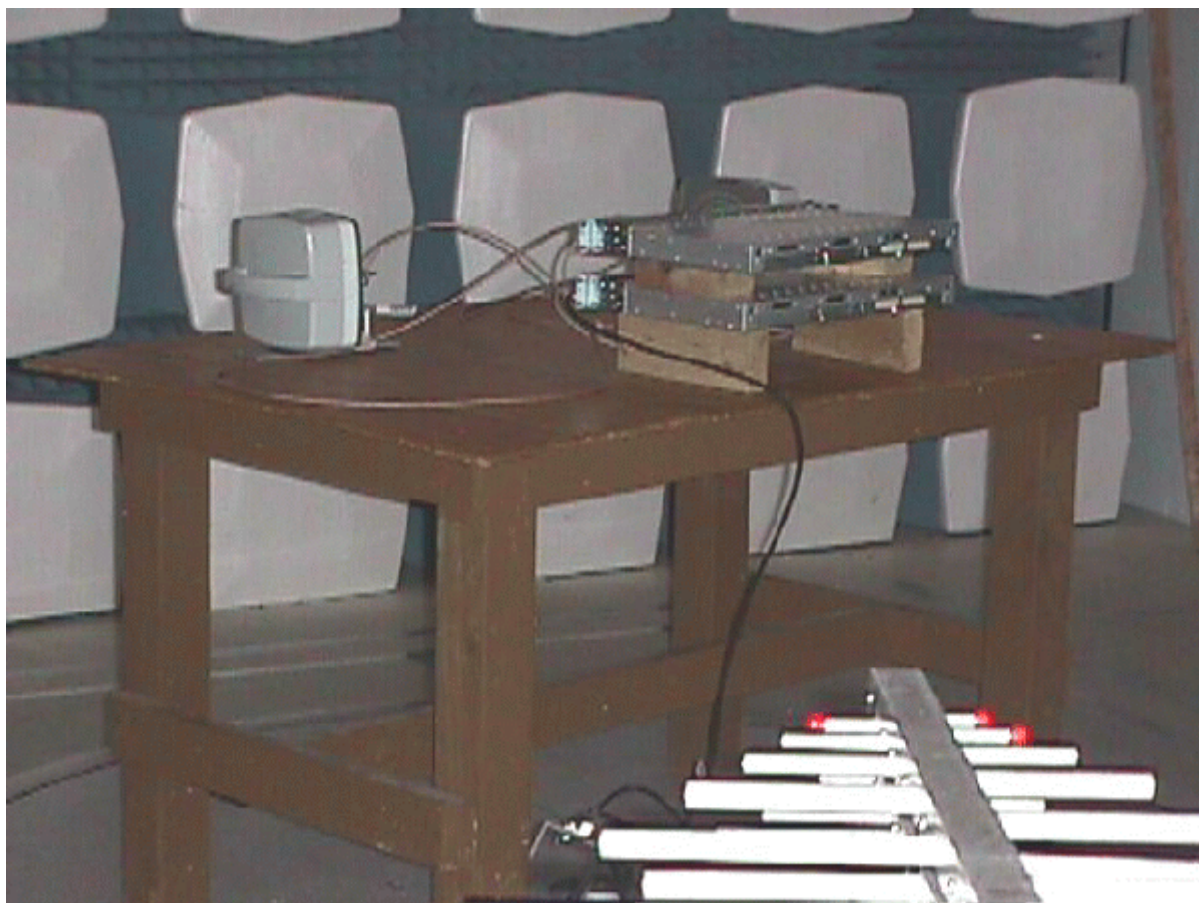
Photograph of Radiated Emissions Test Setup
