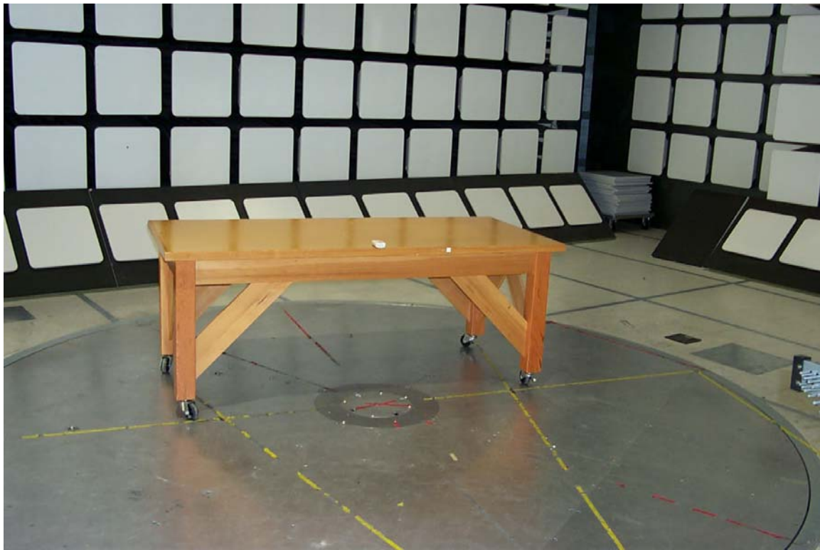
Figure 1 - Radiated Emissions Test Setup
