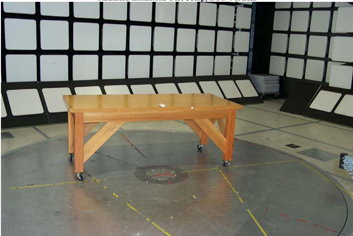
Radiated Emissions Test Setup, EUT Horizontal
