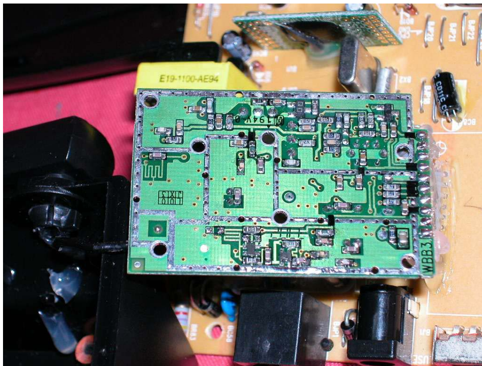
Base Oscillator PCB solder side
