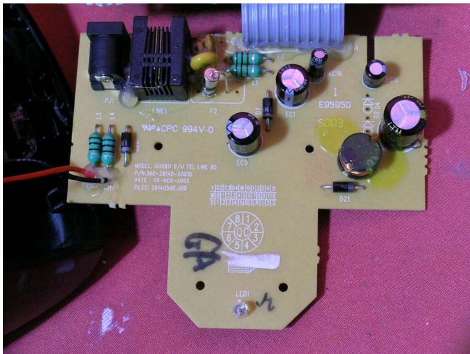
Base Line Interface PCB comp side
