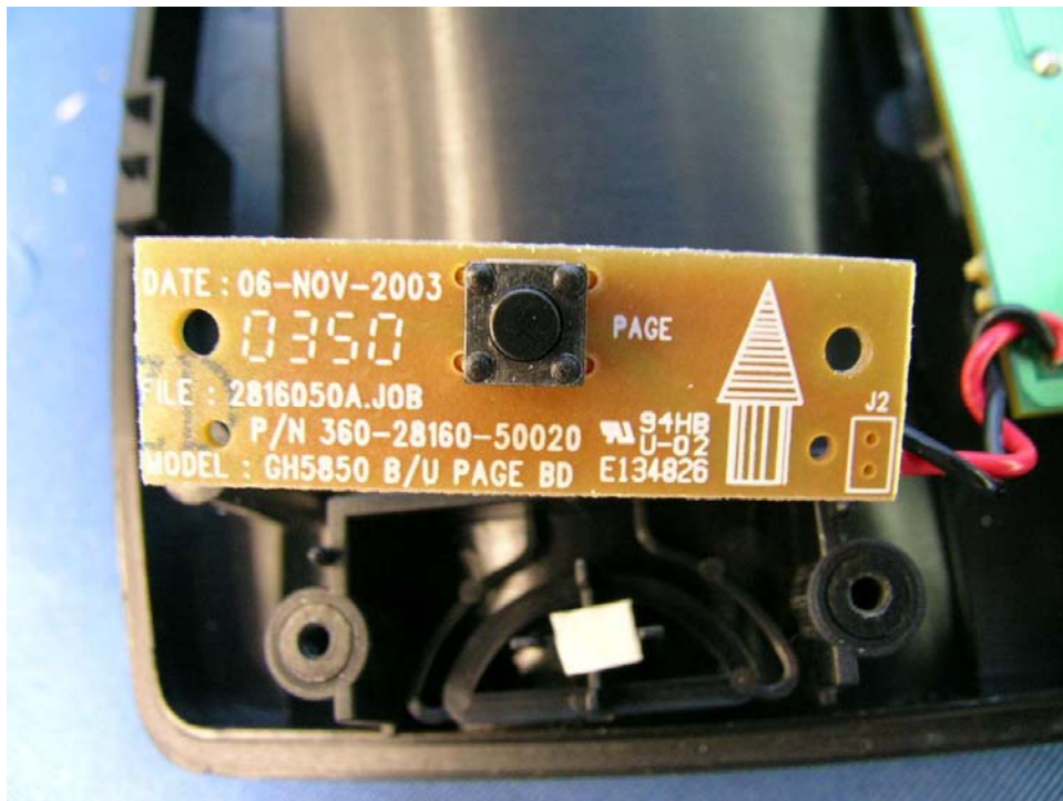
Base Page key PCB front side
