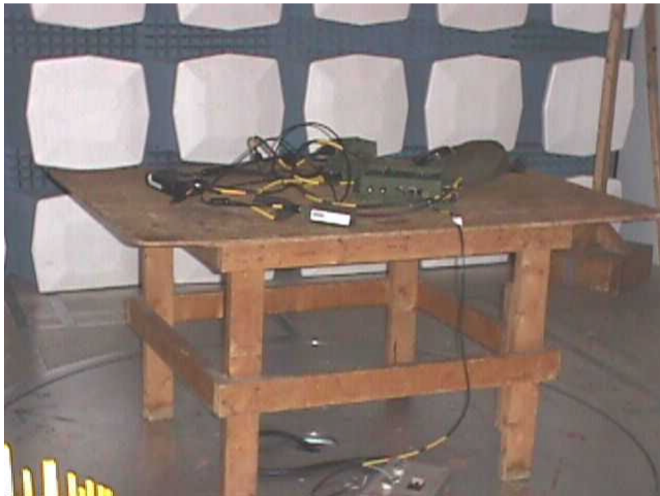
Figure 3. FCC Intentional Radiators Test Setup Photo
