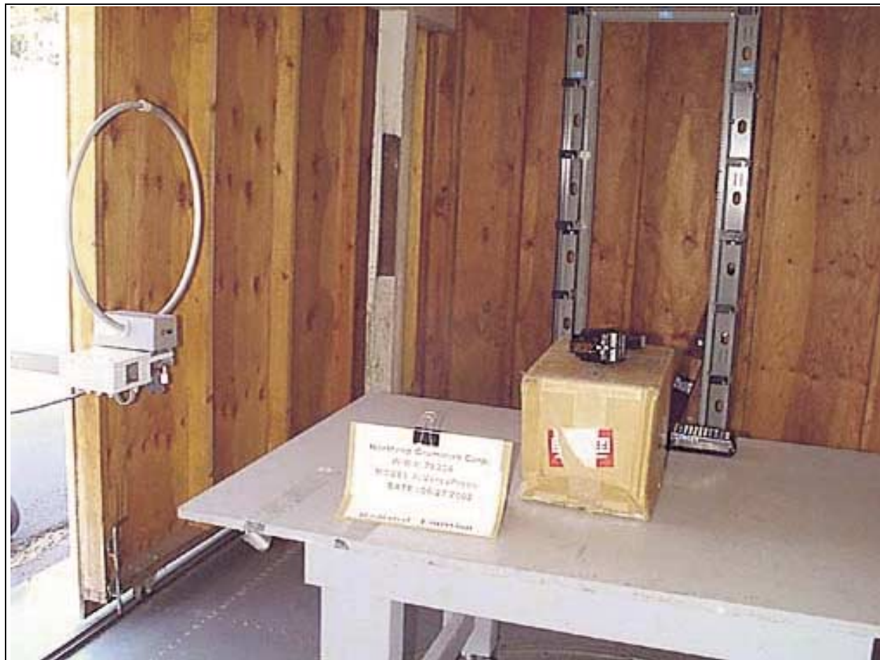
Radiated Emissions - Front View - Loop Antenna
