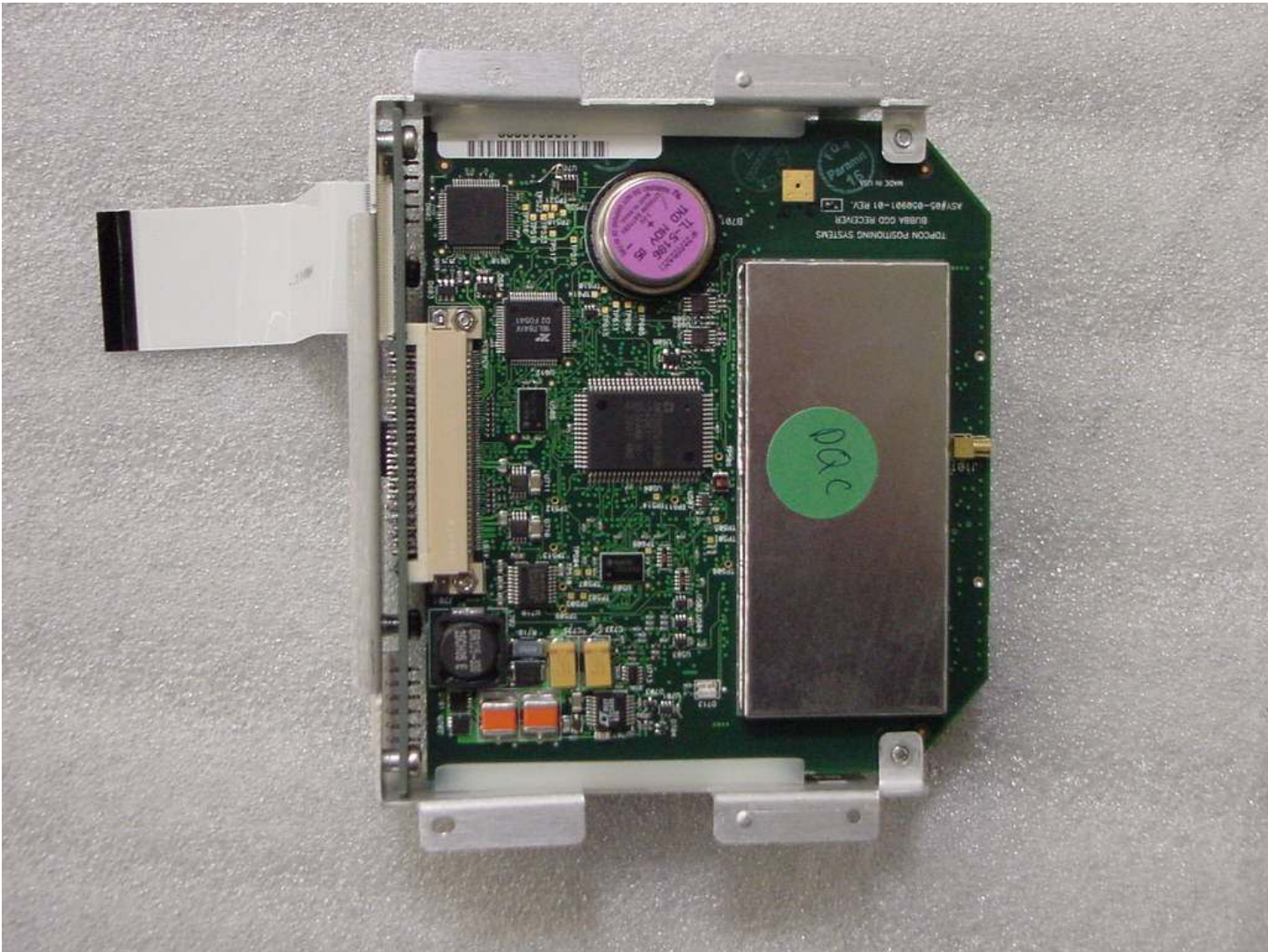
Card cage showing GPS board
