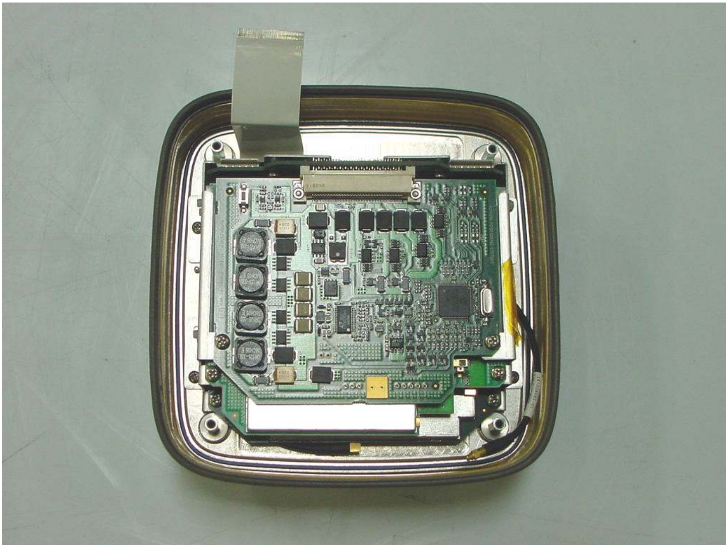
Bottom of card cage assembly showing powerboard
