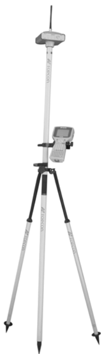
Figure 3-10. HiPer Lite Rover Station Setup
