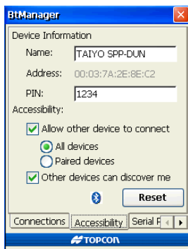
Figure A-2. Check Bluetooth Module Accessibility Settings
