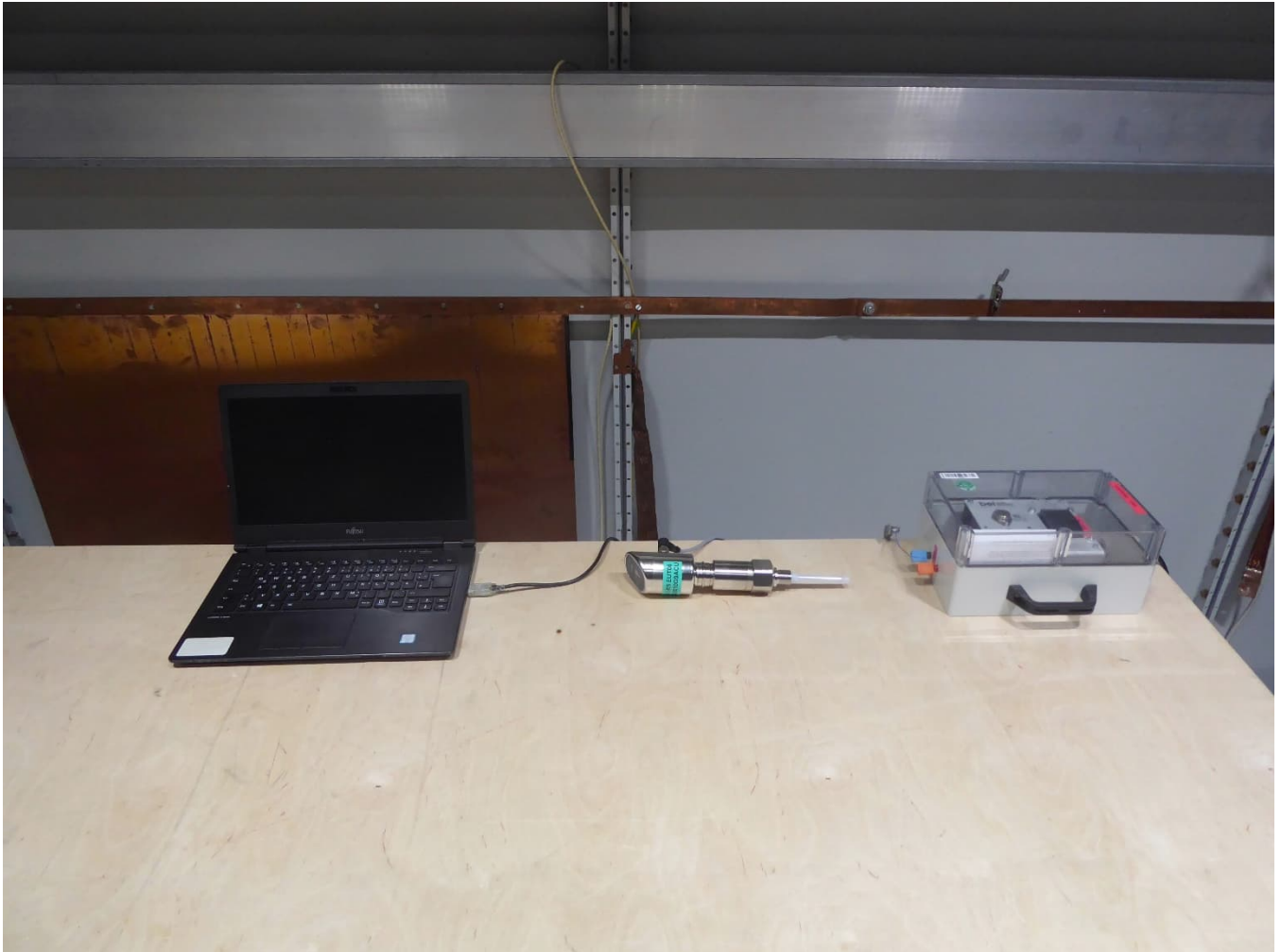
Test setup – AC power line conducted emissions
