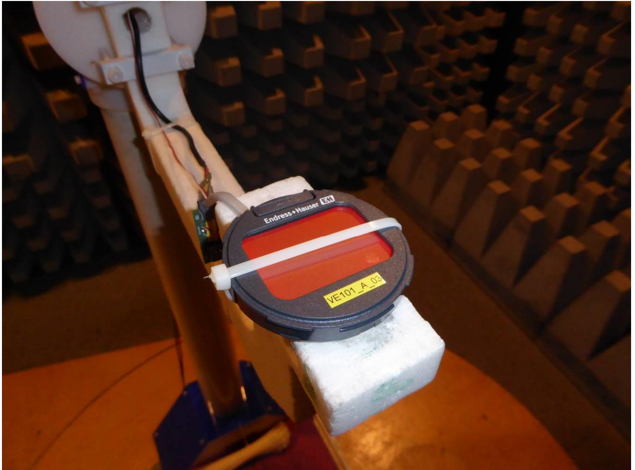
Test setup – radiated test in anechoic chamber
