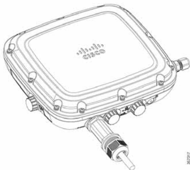
Figure 82: Fiber-Optic cable and gland installed to AP
