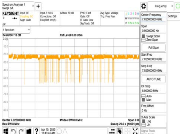
802.11ax_80MHz_CF 7025MHz_ Interference_7025MHz_-76.52dBm_Normal
